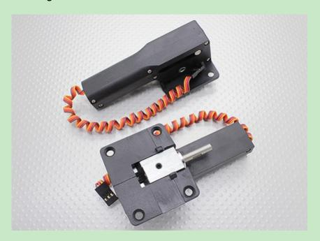
The other frequent breakages are the pins that project from the mechanism and go into the legs. However Mark says in some ways this is good as they provide a weak link and prevent worse damage elsewhere. They are easily replaced.
