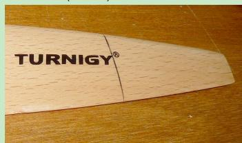
"The reason we measure pitch at 75% of the diameter is two-fold. Generally, the pitch of a propeller is not completely constant,
